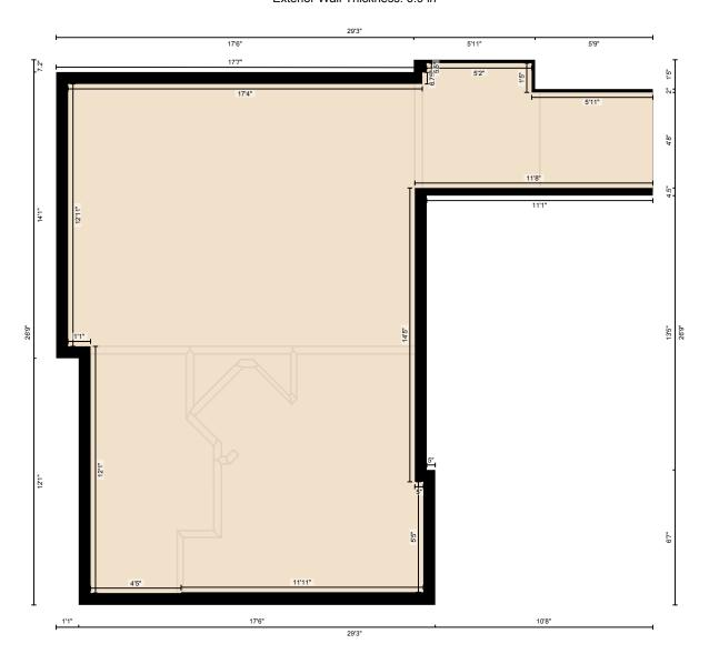
Measurement Diagram for: Basement Exterior Wall Thickness: 7.0 in
