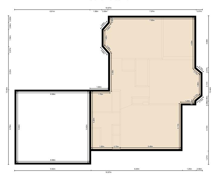
Measurement Diagram for: Upper Floor Exterior Wall Thickness: 17 cm
