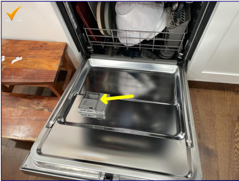
The soap door did not operate properly. Recommend an appliance technician evaluate and repair.
